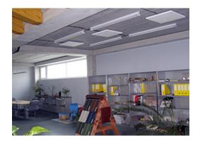
The division of the indoor area into individual offices is executed with the help of light prefabricated partitions which enable future changes to be made in the dispositions of the individual rooms in the building in case of need. This is also one reason why direct-heating ECOFLEX convectors were chosen: they are easy to demount and can be moved to a different location if needed or replaced by a different wattage.
