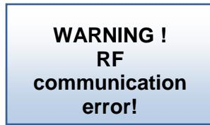
This message will be sent when RF communication is lost between V24 Central and RF antenna of GSM module.
