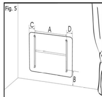
Move the mounting frame up the wall so that the bottom openings in the frame are over the wall-plugged holes labeled “A” - see Fig. 3 and 4 (2). Drill the top holes and insert wall plugs into them. Screw on the mounting frame using screws.
