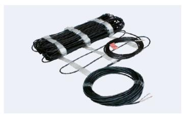
► ADSV+ heating cable - a two-conductor cable with a full protection screen. The sheathing of the cable is resistant against UV radiation and is intended for floor heating and the removal of snow and ice from roofs and eaves troughs.  $1\times3\,\mathrm{m}$  cold lead.  $\varnothing$  5.0 mm. 230 V.
