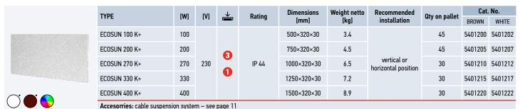
■ Class I.; Basic colour: brown (RAL 8016) thermocrystal surface, white (RAL 9016) gravelly snow surface; Other colours are available to order for an additional fee; Connection cable: 0.75 m for 100-270 K+, 1.2 m for 330-400K+; Bolts and ceiling fixing frame are included in the packing.
