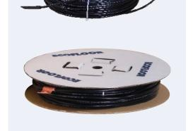
▶ **PSV heating cable** – a single-conductor cable with a full protection screen for storage and semi-storage heating. Cold lead 2×5 m. 230 V. Cable diameter 4.5–4.8 mm.
