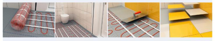
► ADSV heating cable – a twin conductor cable with a full protection screen suitable for wet areas. For direct floor heating or floor renovation (installation under tiles). Cable diameter 3.4–4.2 mm. 230 V. Halogen free cold lead 1×3 m.
