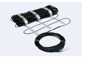
► ADPSV heating cable / mat – a twin conductor, full protection screened cable with protection against UV radiation. This multipurpose cable is suitable for indoor and outdoor applications. Class M2. 1×5 m cold lead. Ø 5.0-5.9 mm. ADPSV heating mat: width 0.5 m. Packed in PE foil.
