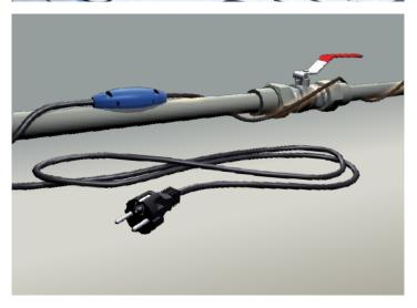
MAPSV heating cable – a single-conductor cable with a full protection screen and protection against UV radiation. Suitable for heating outdoor surfaces. Cold lead 2×5 m. Ø 5.9-6.4 mm. Packed in PE foil.
