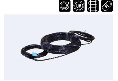
MADPSP heating cable / MDT heating mat - a two-conductor cable with a full protection screen and protection against UV radiation. Suitable for heating outdoor surfaces. Class M2. Cold lead 1×5 m. Ø 6.3–9 mm. MDT heating mat: width 0.75 m. Packed in PE foil.
