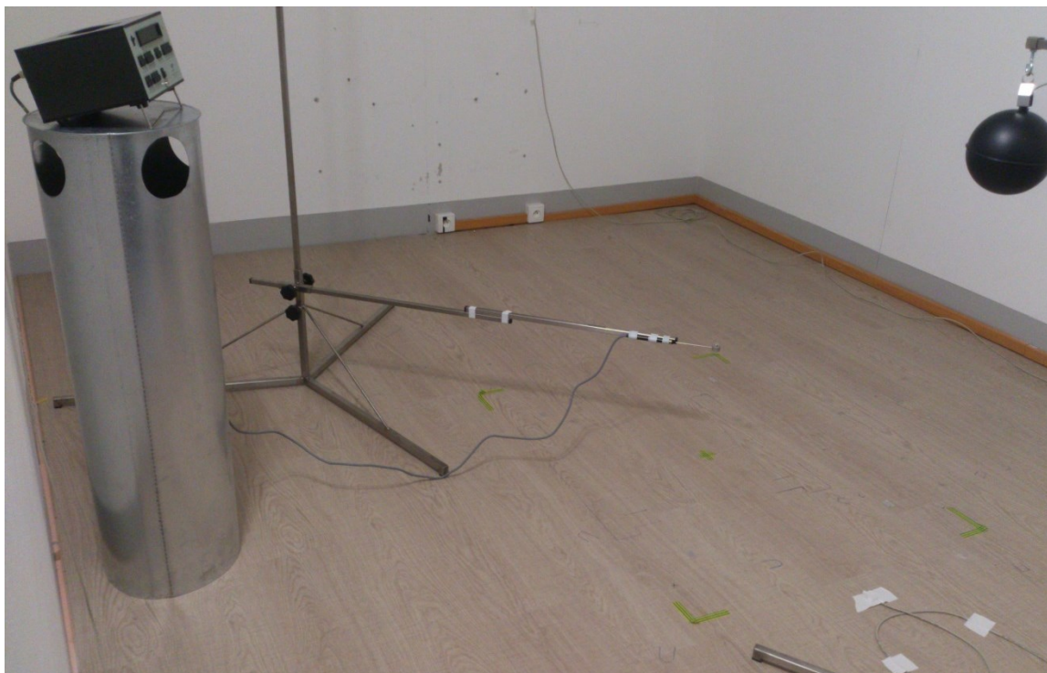
Figure 5-1 View into the measuring chamber ready to measure the heat flux of floor heating. On the left is a datalogger and a sensor for measuring radiant heat flux. On the floor is a length scale for the thermal camera. On the right is a globe thermometer.
