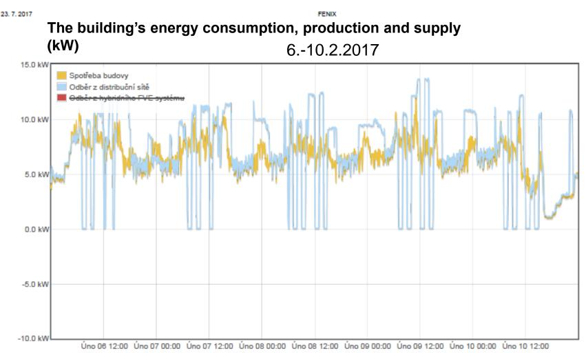
A comparison of the real energy consumption of the building with its energy consumption from the grid shows the ability of the battery storage system to achieve zero consumption from the grid during peak periods (HT) and
