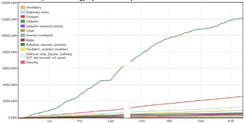
Electric heating had a significant share in the energy consumption during the heating period, amounting to 59.8% of total consumption.
