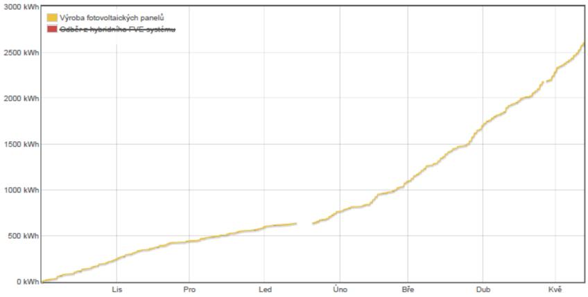
The photovoltaic panels produced 2 507 kWh during the heating season, i.e. 12.5% of the total energy consumed
