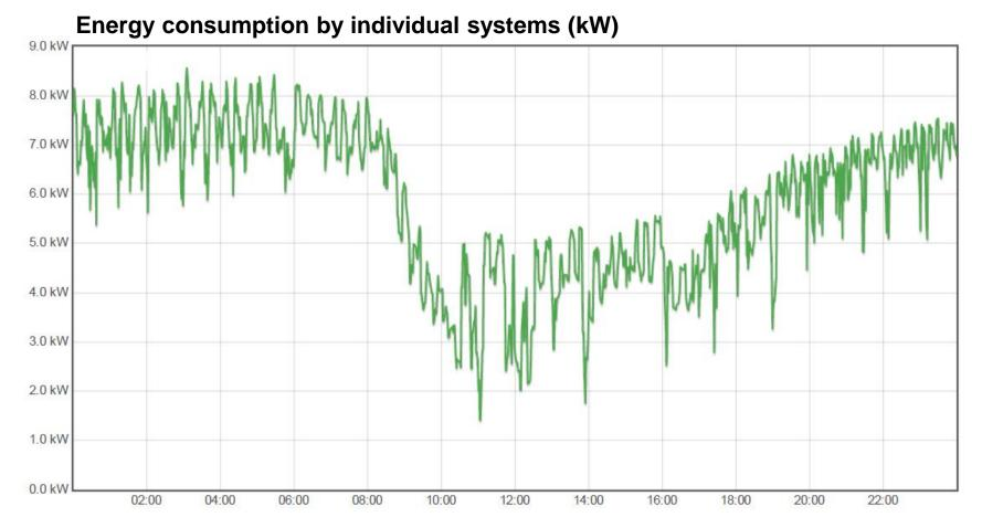
The energy consumed by heating (radiant heating system) reacts flexibly to the changes in outdoor temperatures and mainly to random heat gains (people – technology)
