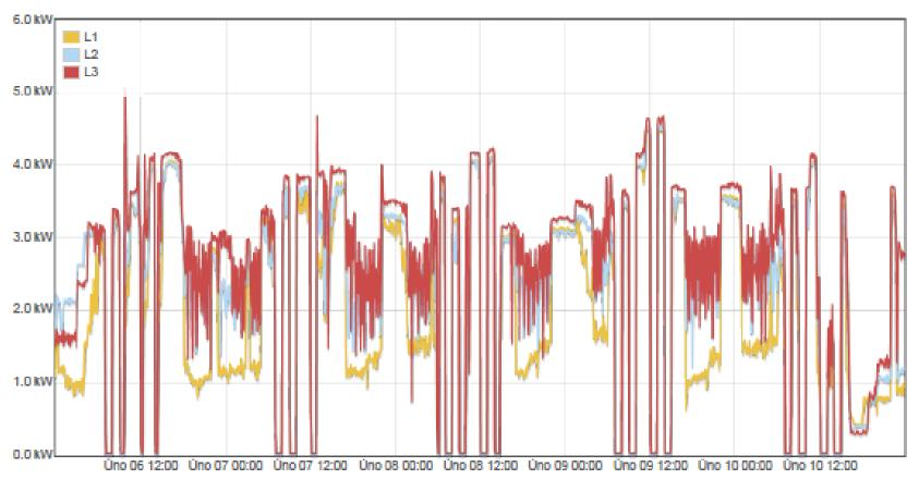
The storage system contributes to the even distribution of consumption in the individual phases. In the zero consumption mode, it reliably ensures zero consumption in all phases.
