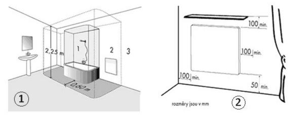
During the installation of radiant heating panels, the following minimum clearances must be observed (Pict.2):
