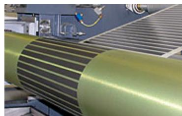
The production technology allows the production of heating foil with a width of 300mm to 1200mm, for a voltage of 12V to 230V and theoretically, with any output from 20 to 300 W/m<sup>2</sup>. In the interests of production efficiency, it is necessary to produce approximately 1000m of foil of one type in one production ‘run’. Therefore, it isn’t possible to produce the foils on demand as a standard service, and they are offered only in standardized outputs and widths.
